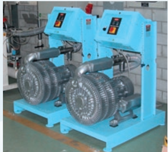
Battery of pumps with side channels. Bateria de bombas com canais laterais.
